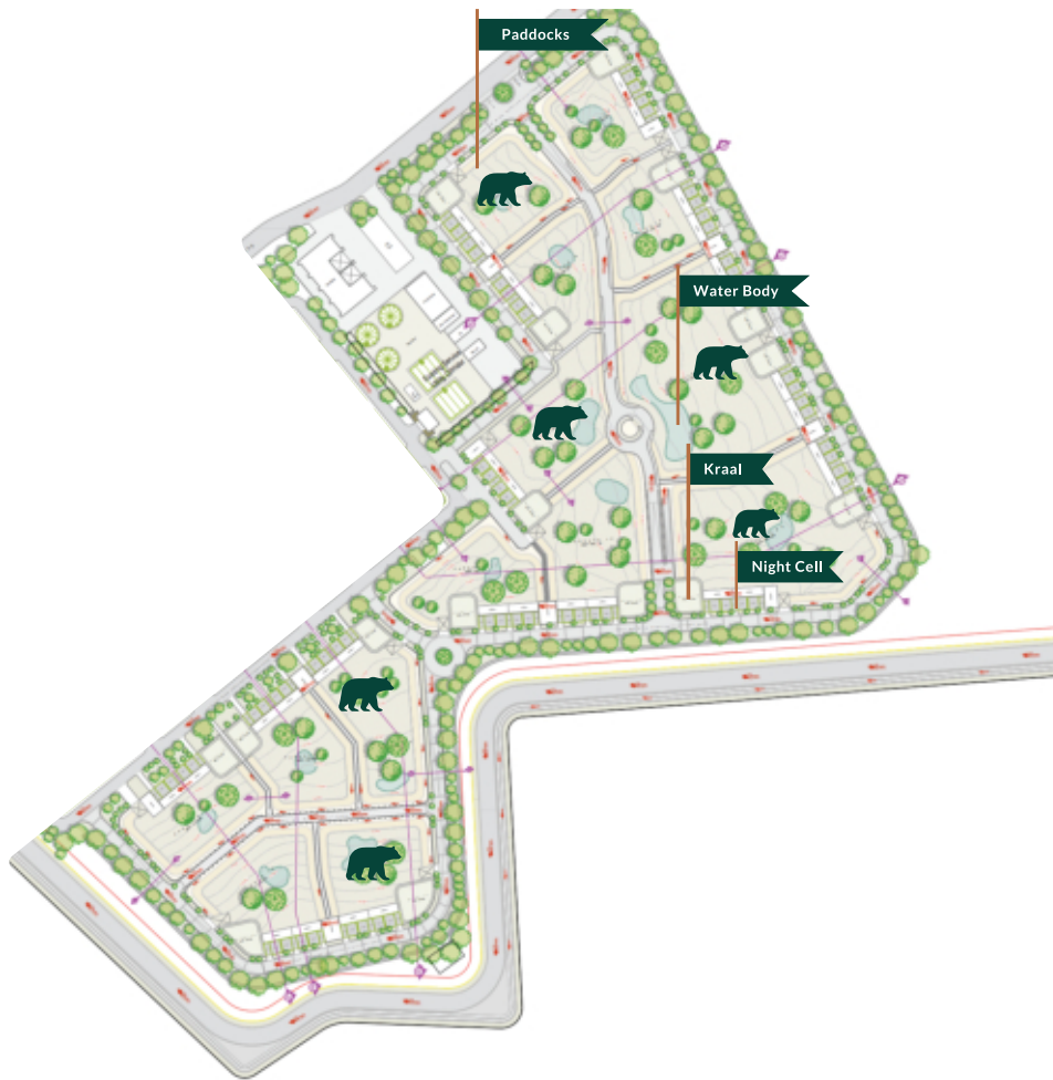
Layout design of the Bear Extension Facility, illustrating the arrangement of paddocks, night cells, kraals, and enrichment zones for optimized bear welfare and management at GZRRRC.
